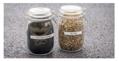
It is the first-time bitumen modified with waste tyre material – which included the equivalent of 40,000 beer bottles of recycled glass, as well as the end-of-life truck tyres - has been used in Tasmania.
