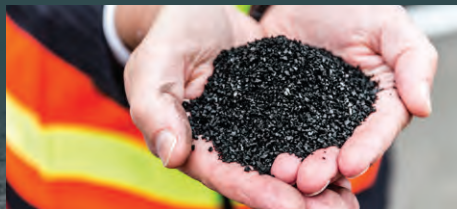
Recycled crumbed rubber granules - a valuable recycled raw material that Tyre Stewardship Australia is working to find more uses for.
