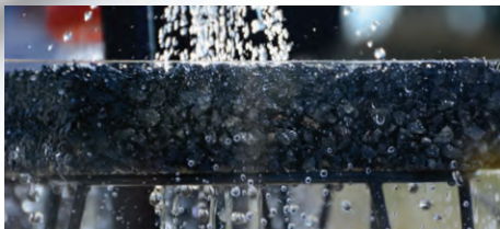
From top: 1. Use of recycled tyre rubber granules in synthetic sporting fields and pitches provides a stable, shock absorbing and durable base layer. 2. Development of reinforced concrete - using baled end-of-life tyres sandwiched between highly stable concrete skins, for use as retaining wall or blast resistant wall. 3. A series of blast tests on an innovative product aimed at making walls blast, bullet and fire-resistant using a combination of recycled crumb rubber from old tyres with composite fibres in a cementitious mix design. 4. Crumb rubber permeable pavement installed at St Mary's Park in the City of Mitcham SA. This is the first time permeable pavement, made using 50% used tyres, has been installed in a full-scale trial tested under various traffic loads.
